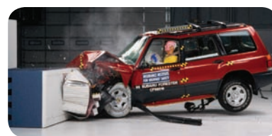
FIGURE 6.4 (Example 6.2) (a) This car's momentum changes as a result of its collision with the wall. (b) In a crash test (an inelastic collision), much of the car's initial kinetic energy is transformed into the energy it took to damage the vehicle.
